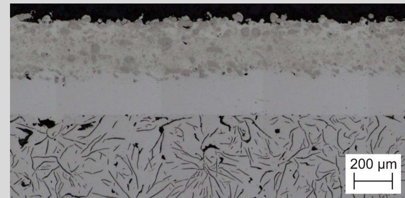
32/32/24/23 g/min AISI 430L 21/13 g/min TiC/FeCr 70/30
