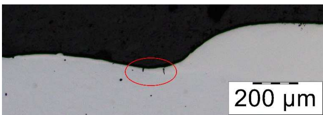
Figure 7: Cross section image of a single FeCrNiB bead on a E235+C tube substrate deposited at a surface speed of 20 m/min with crack nuclei at the fringes.
