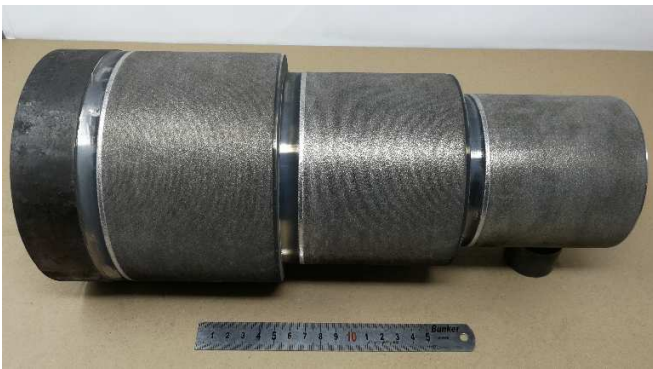
Figure 6: Duplex steel claddings on a S355 shaft substrate with sections showing diameters of 150, 125 and 100 mm.
